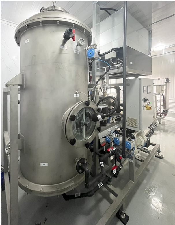
The emulsion concentration system recovers 80 cubic metres of water that can be used for cooling purposes.
